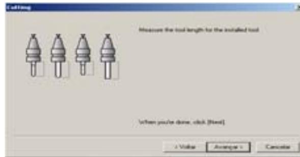
7) The tool length should already be measured with the machine, if so skip to 11). If not: click on [Magazine].
