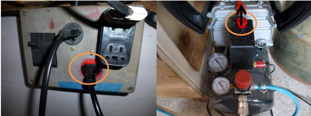
1) Plug in the handypanel. (To remove the handypanel it is important to not pull the plug out without pulling the security which is around it!)
