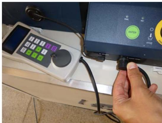
2) Start the machine by pushing the button at side of the front panel. Nothing happens: check if the emergency stop is not pressed and the electricityplug is connected.
